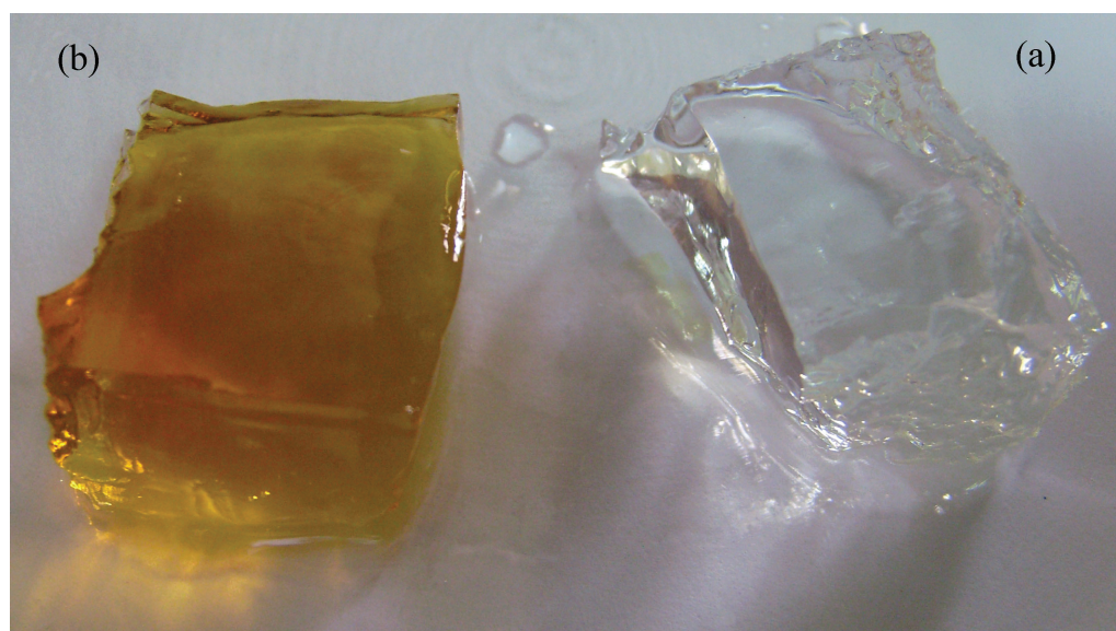
Fig. 1. Photographs of (a) dextran hydrogel, and (b) dextran hydrogel-silver nanocomposites.
